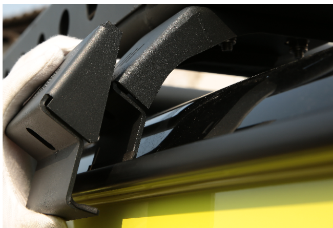
Gutter supports clamped onto the roof rain gutter.
