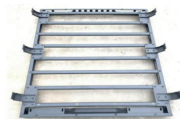
Inner support brackets fitted to the rack, and all 6 brackets installed.
