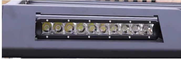
LED light bar seated in the front rail cutout.
